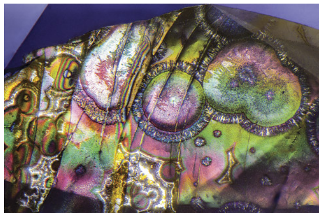
Figure 9. Radial limonite within a surface-reaching fracture of a violet sapphire shows bright interference colors when viewed under diffused reflected light. Photomicrograph by Nathan Renfro; field of view 1.44 mm.
