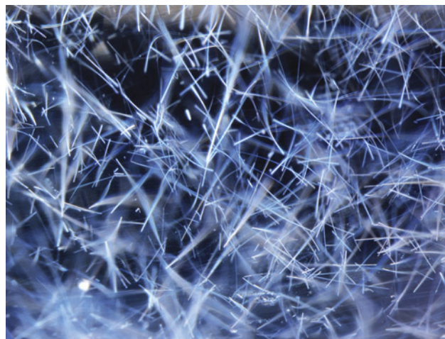
Figure 2. Whitish hairlike inclusions in a 3.55 ct faceted benitoite. Photomicrograph by Taku Okada; field of view 2.37 mm.
