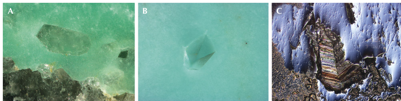
Figure 10. Euhedral quartz crystals in turquoise. A: Quartz with a hexagonal prism cross section (perpendicular to the c-axis). B: Quartz with a pyramidal trigonal habit. C: Quartz showing transverse striations under differential interference contrast microscopy. Photomicrographs by Ling Liu; fields of view 0.9 mm (A), 0.5 mm (B), and 0.6 mm (C).
