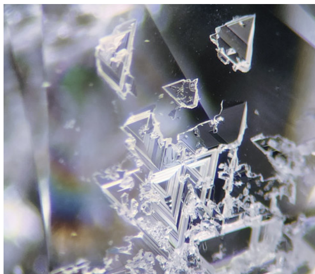
Figure 4. A collection of trigons on the pavilion surface of a round brilliant-cut diamond. Photomicrograph by Isabelle Corvin; field of view approximately 2.0 mm.
