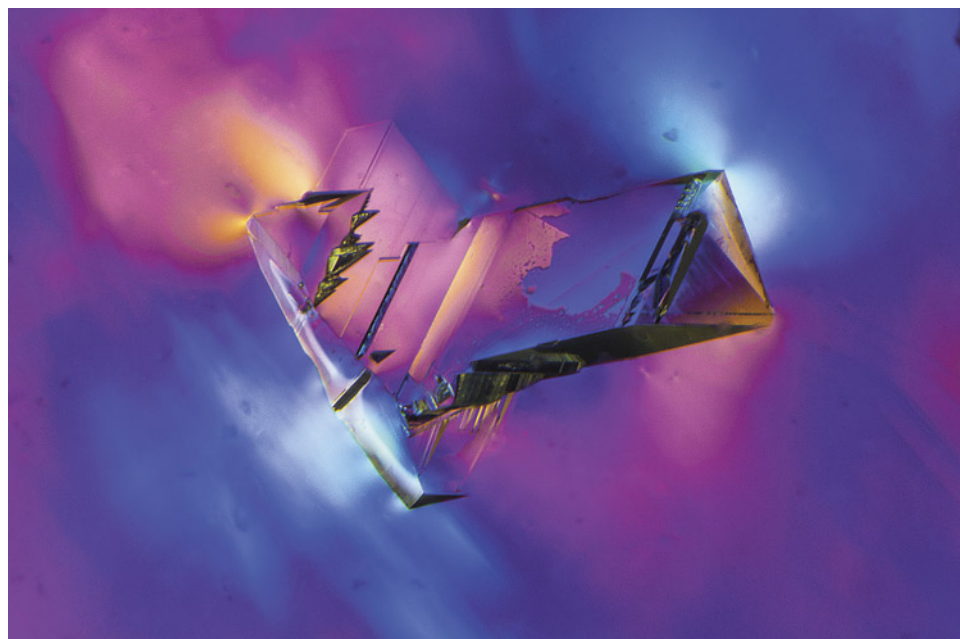
Figure 18. Polarized light shows an elongated modified diamond octahedron displaying various degrees of interfacing with the host diamond crystal. Photomicrograph by Nathan Renfro; field of view 2.18 mm.
