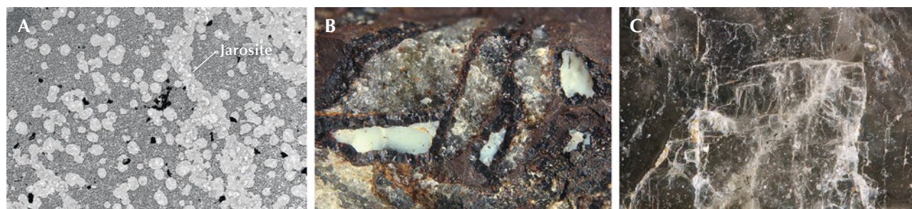
Figure 17. A: Jarosite has the brightest gray value in this BSE image. B: Bonattite with a milky appearance filling in the fissures and wedge-shaped cavities of goethite. C: Muscovite with perfect cleavage, found in the matrix of rough samples. Photomicrographs by Ling Liu; fields of view 1.2 mm (A), 5.9 mm (B), and 1.1 mm (C).
